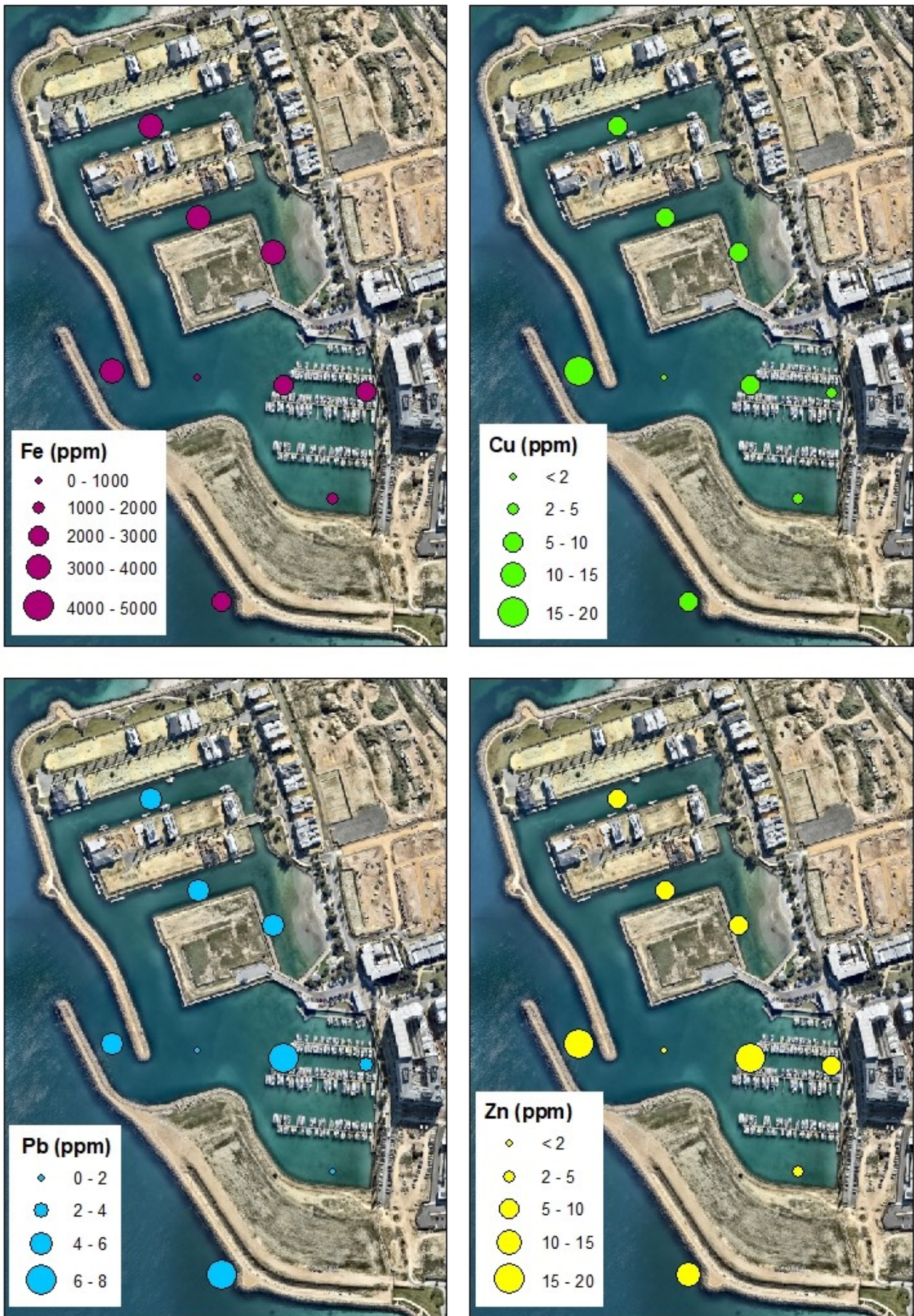
Figure 7: Cartogram for Iron (Fe), Copper (Cu), Lead (Pb) and Zinc (Zn) at 9 locations at the Port Coogee Marina (March 2019)
