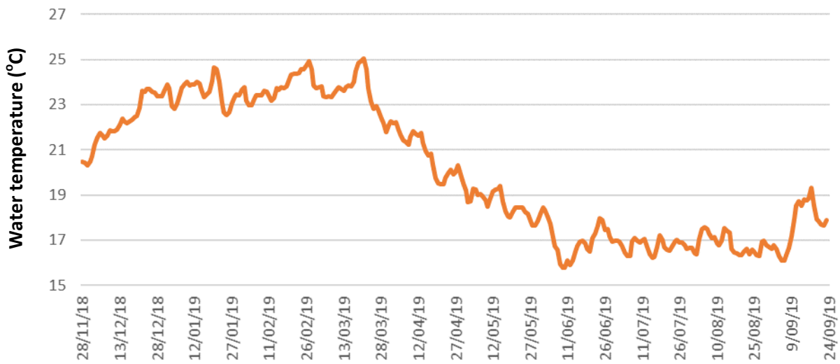
Figure 5: Daily average water temperature from 3m depth in Port Coogee Marina (location Fig. 1)
