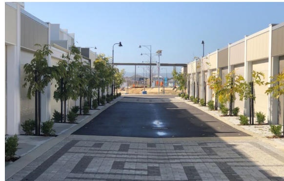
Figure 4. Staggered trees in a rear laneway, Treeby, demonstrating how keeping services out of the laneway provides these opportunities
