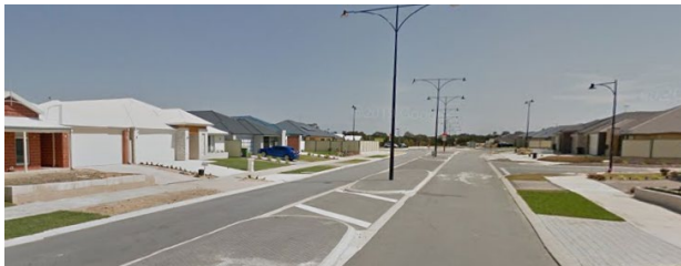
Figure 8. Residential streetscape in Hammond Park where hardscaping dominates due to insufficient space for street trees and numerous breaks in the median for access to crossovers
