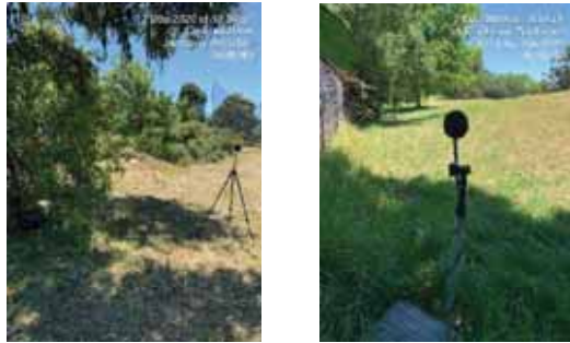
FIGURE 3.2 - NOISE MONITOR IN SITU
