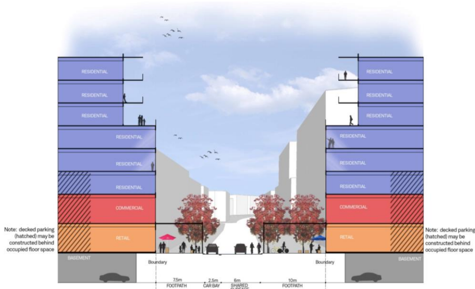
Figure 05_Typical cross section for activity centre development
