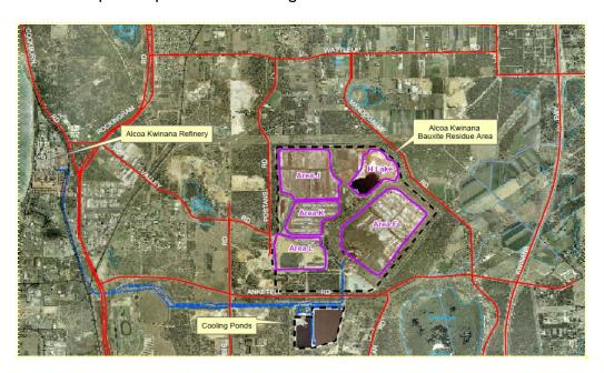
The residue product itself is made up of two components of roughly equal quantity - sand and mud. Much of the sand is reused for construction of, and within the residue drying areas. The residue mud is dried in layers, with layers incrementally built up with mud to create residue stacks.
