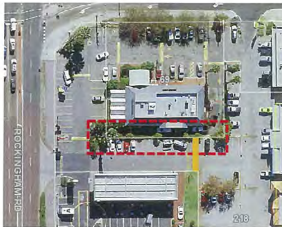
Figure 20. Northern end parking bays for re-consideration, orange line showing where access was intended to be blocked
