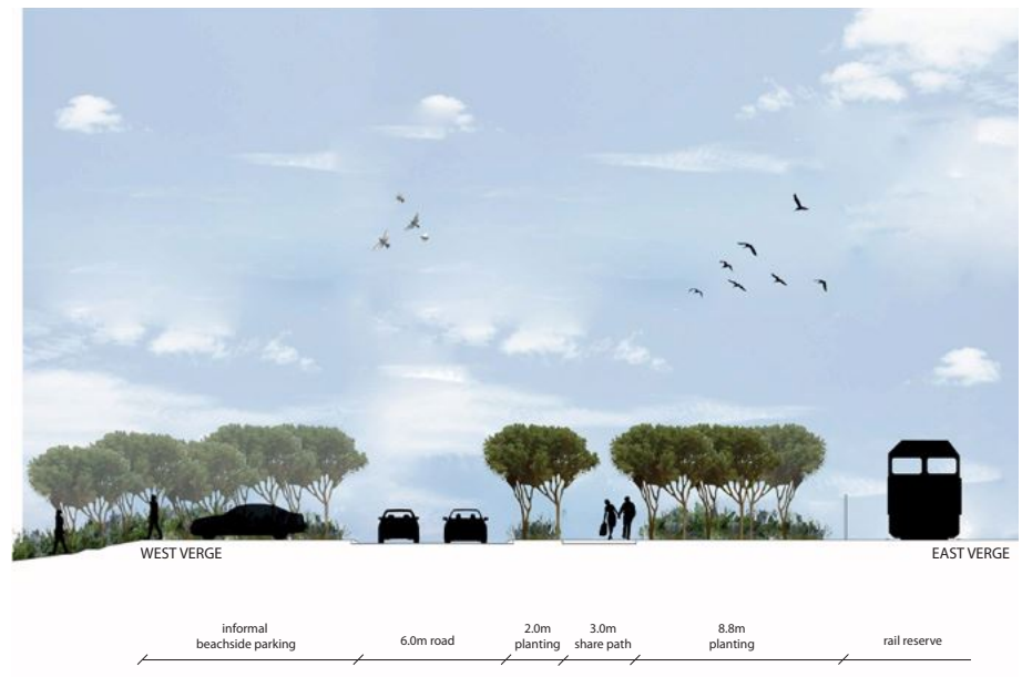
Robb Road Local Street - Typical Section
