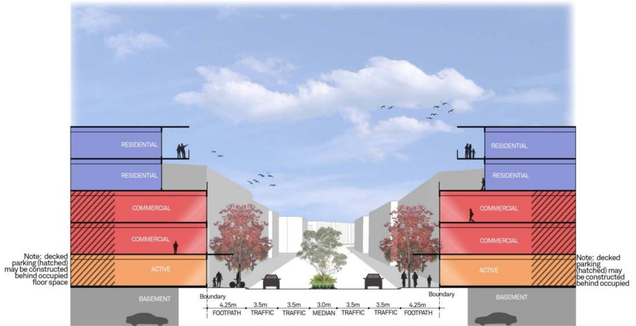
Figure 07_Typical cross section for mixed use development
