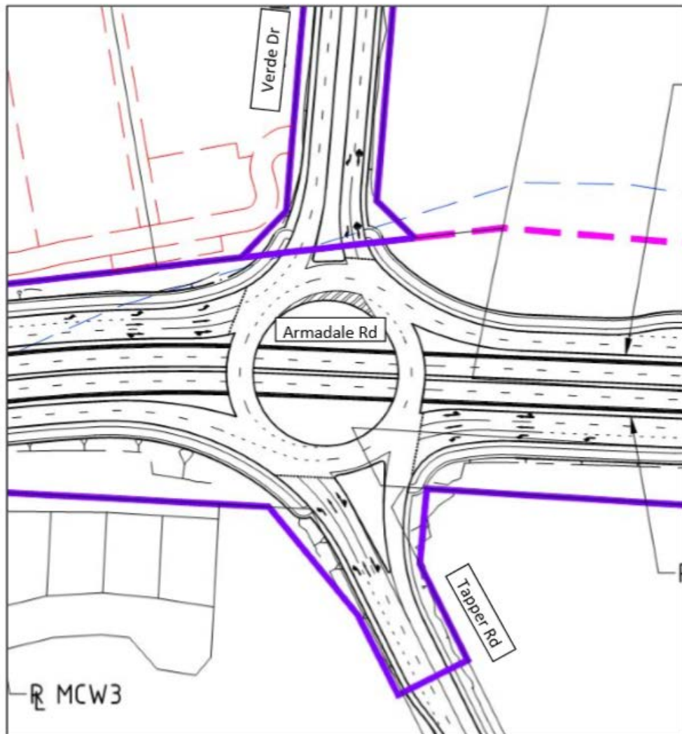
Figure 42 Armadale Road/Tapper Road/Verde Drive Intersection Layout
