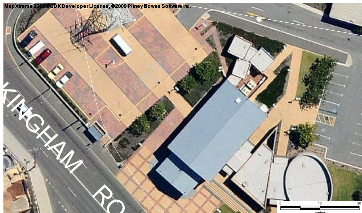
Aerial 3. The broad paving stripes in this car park at the Memorial Hall, Rockingham Road, Hamilton Hill, create the sense that this car park is a pedestrian space. Had it been asphalt with white line markings the space would lose its identity and be indistinguishable for the streets and roads around it.
