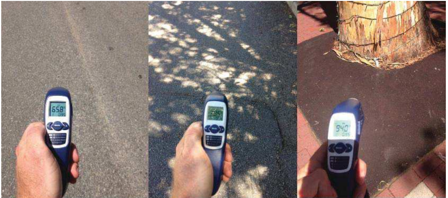
Bitumen in full sun= 65.8°C
