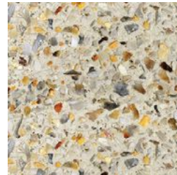
shared path_ washed aggregate concrete
