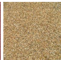
surface treatment_ stabilised gravel
