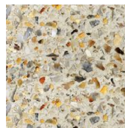
shared path_ washed aggregate concrete
