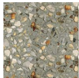
shared path_ washed aggregate concrete
