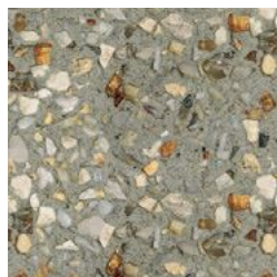
shared path_ washed aggregate concrete
