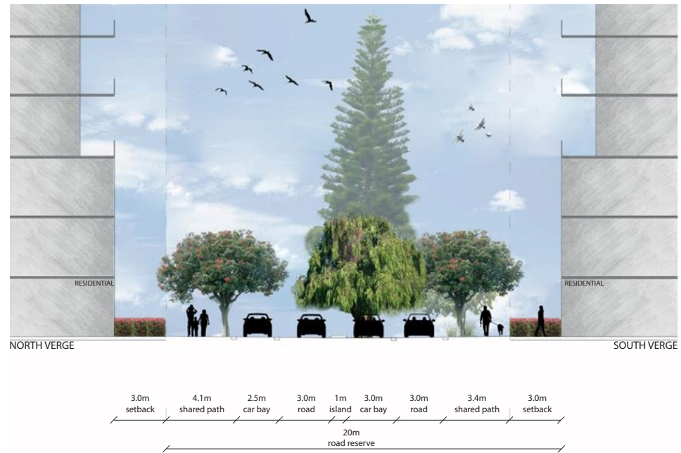
Emplacement Crescent Shared Street 1 - Typical Section
