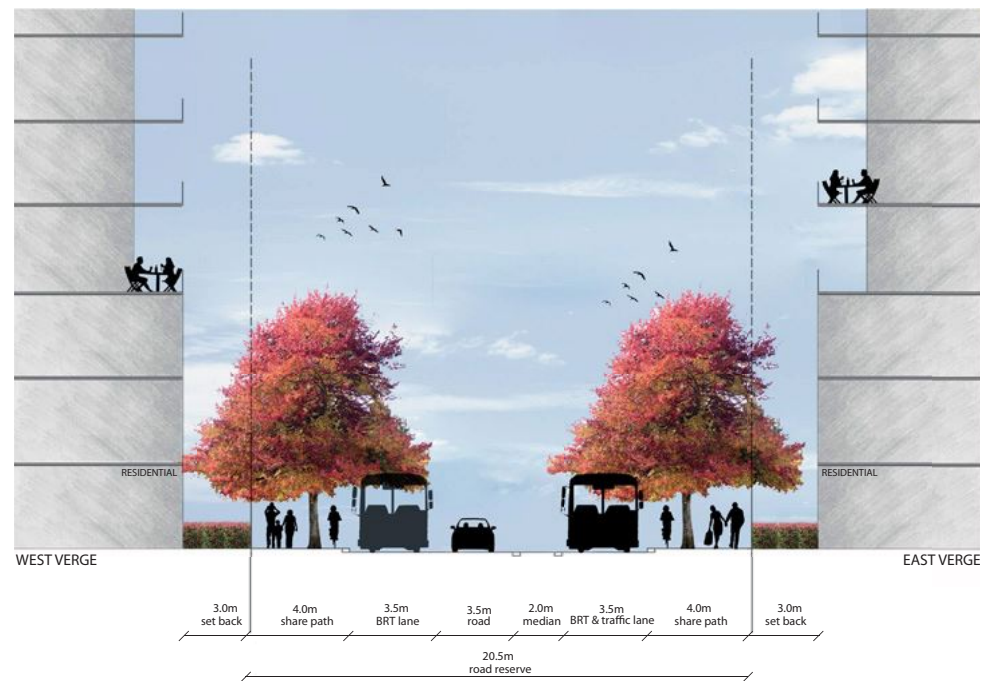
BRT Local Road_Residential Zone - Typical Section
