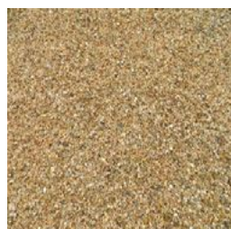
surface treatment_ stabilised gravel
