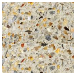
shared path_ washed aggregate concrete
