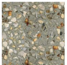
shared path_ washed aggregate concrete
