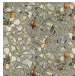
shared path_ washed aggregate concrete
