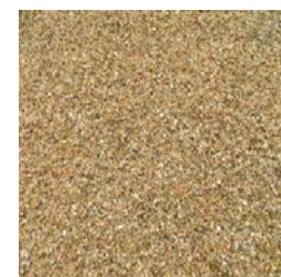
surface treatment_ stabilised gravel
