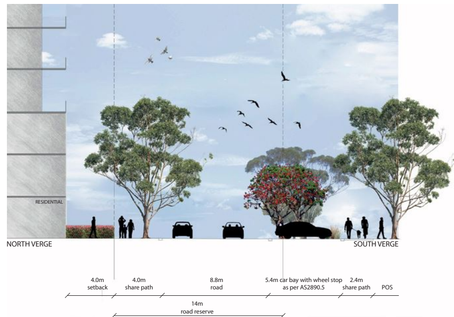
POS Street - Typical Section
