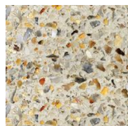
shared path_ washed aggregate concrete
