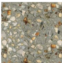
shared path_ washed aggregate concrete
