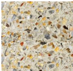
shared path_ washed aggregate concrete
