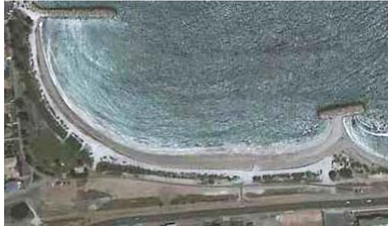
Figure 4 Detached breakwater (bottom right) forming a tombolo in Geraldton, Western Australia, as part of a coastal protection and harbour configuration (Source: Google Earth)
