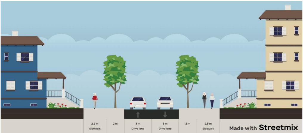
Figure 12 Indicative Cross Section – Road 1
