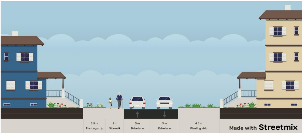
Figure 13 Indicative Cross Section – Road 2
