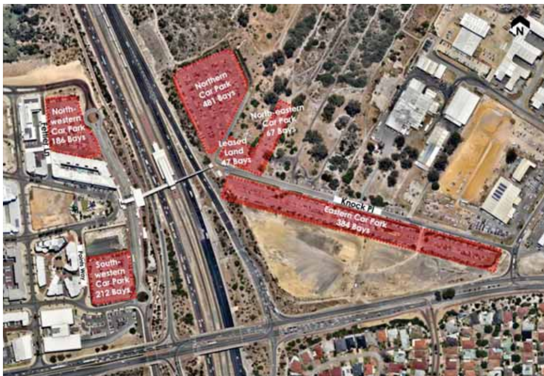
Figure 2.5: Existing Location and Number of PTA Car Parks Associated with the Cockburn Central Station
