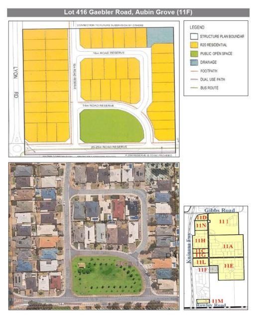
Located at the southern end of the main residual portion of DA11 along the eastern edge of Lyon Road, this Structure Plan identifies a local road network servicing low density (R20) housing focussed around a surrounding a southern POS reserve (Bologna Park).
