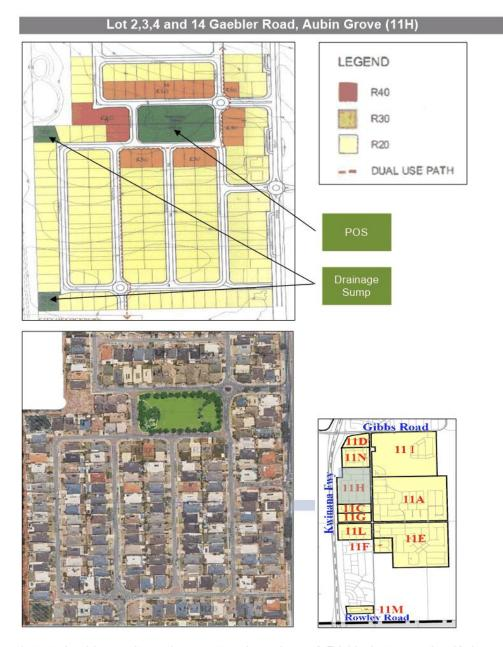
Located midway along the western boundary of DA11, between the Kwinana Freeway and Lyon Roads, this structure plan identifies a local road and drainage network principally servicing low density (R20) housing, with medium density (R30 and R40) housing immediately surrounding a northerly centralised POS reserve (Bologna Park).
