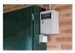
Main monitoring hub accessible through a secure web interface
