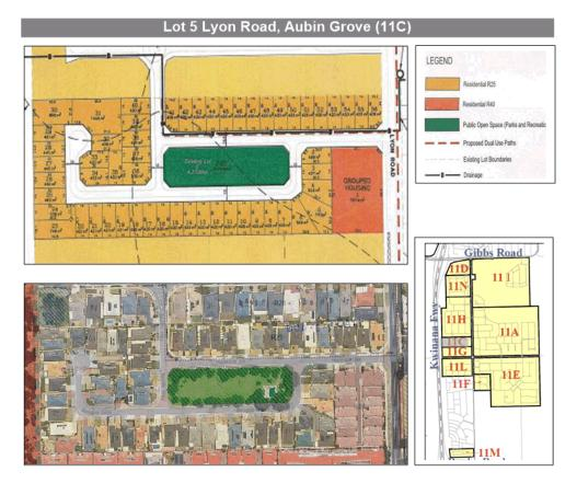
Located midway along the western boundary of DA11, between the Kwinana Freeway and Lyon Road, this structure plan identifies a local road and drainage network and low density (R25) housing around a central POS reserve (Bologna Park).
