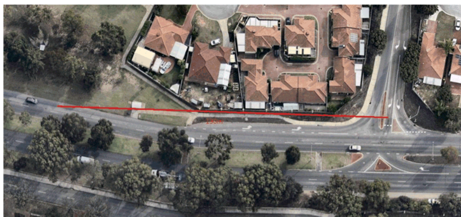
Figure 1: Available Intersection Sight Distance (130m)
