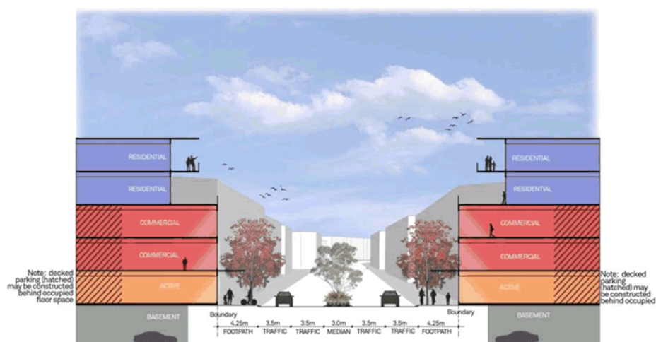
Figure 07/_ Typical cross section for mixed use development
