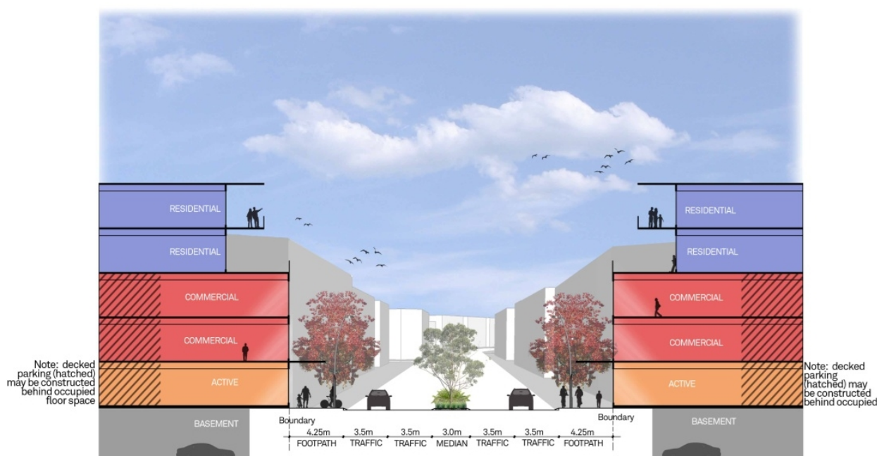
Figure 07_Typical cross section for mixed use development
