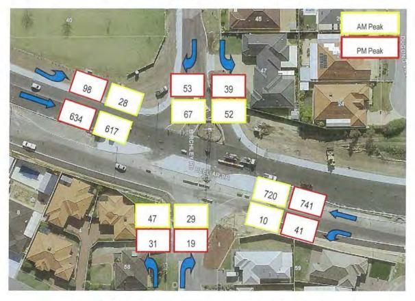
Figure 8 - Existing Peak Hour Flows on Beeliar Drive / Birchley Road intersection
