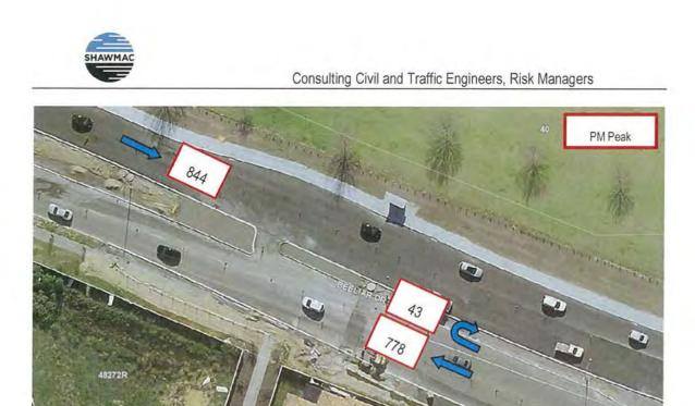
Figure 10 Predicted Peak Hour Flows on the U-turn pocket
