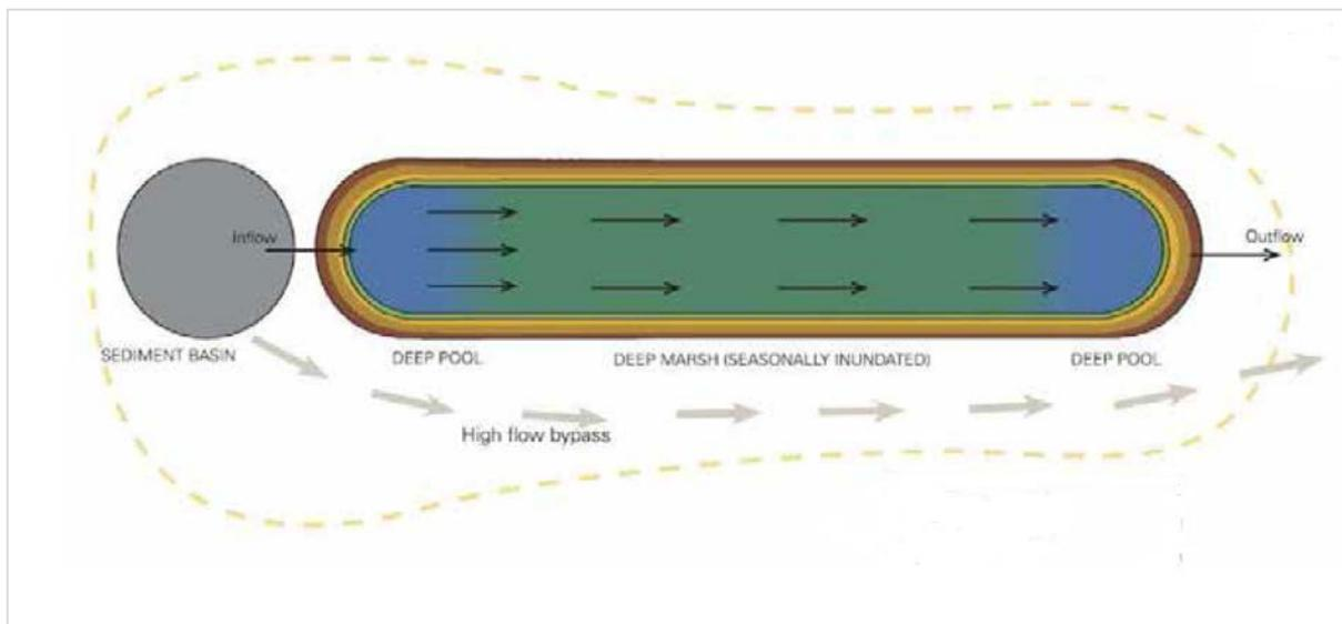
**Plate 3 Typical Constructed Wetland Layout**
