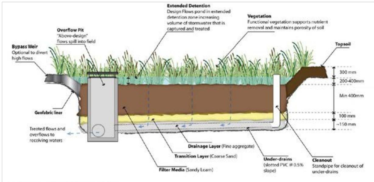
**Plate 2 Typical Bioretention Basin Layout**
