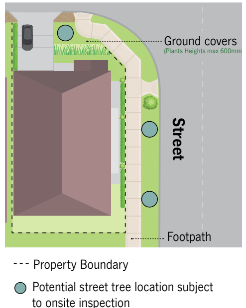
Figure 3. Corner block narrow verge design.
