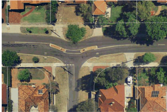
Figure 4 – Typical T-Junction Slow Point Installation
