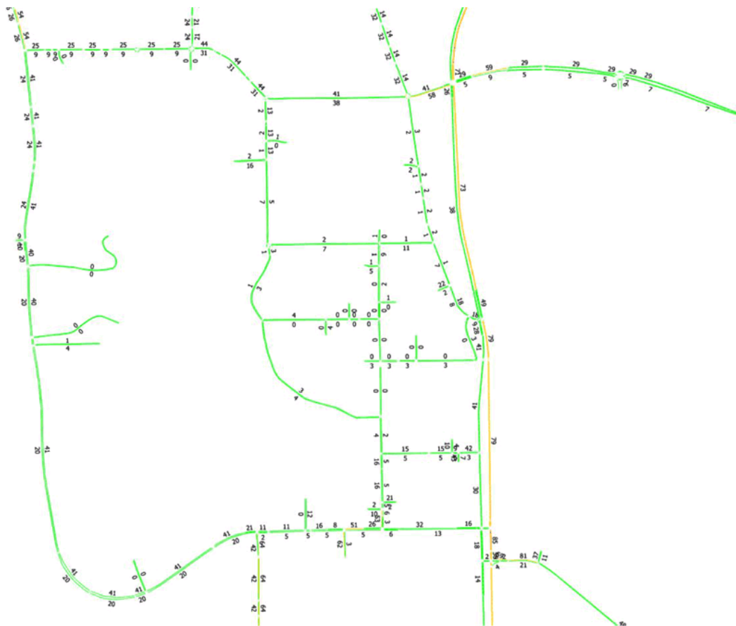
Figure 6 – Volume capacity ratio PM peak period (16:00-18:00), Fawcett Road open (Note: Values are in %)
