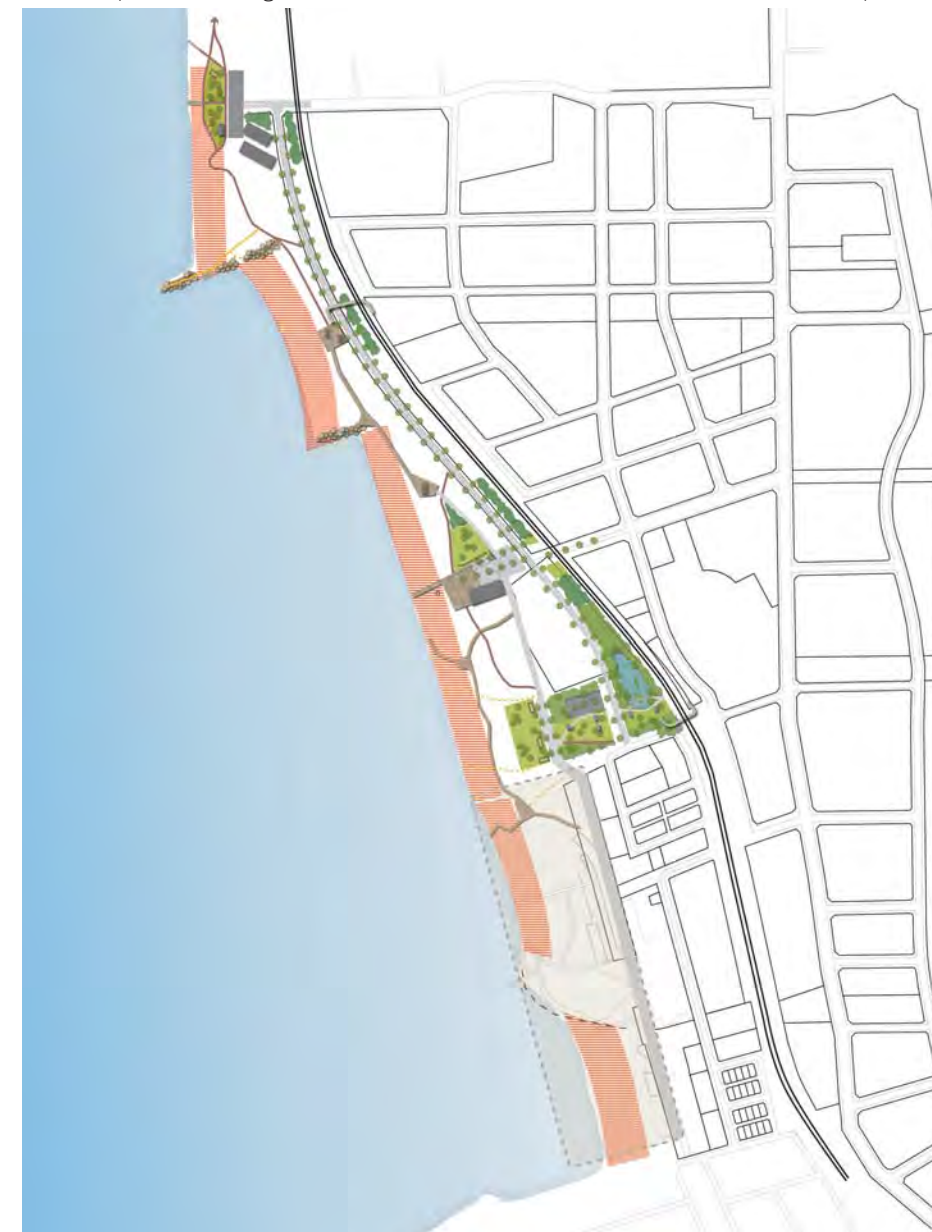
Figure 5.14 Infrastructure and Facilities - Groyne and Nourishment Option
