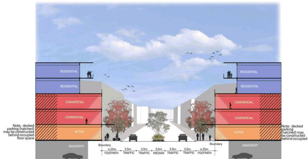
Figure 07_Typical cross section for mixed use development
