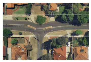
Figure 4 – Typical T-Junction Slow Point Installation
